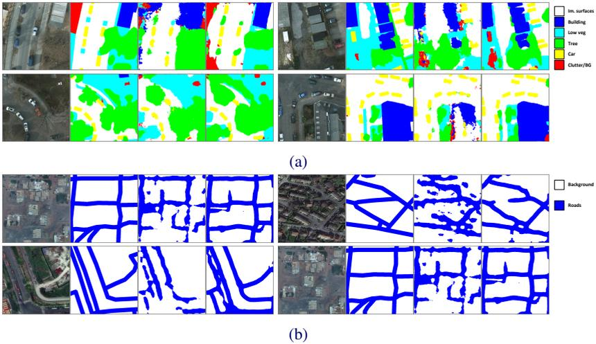
Figure 5: Qualitative semantic segmentation results for Potsdam (a) and SpaceNet Road (b), from left to right: input image, ground truth, prediction with model trained from scratch, and prediction with model pre-trained using our approach. 10% of labeled data is used for fine-tuning in all cases.
